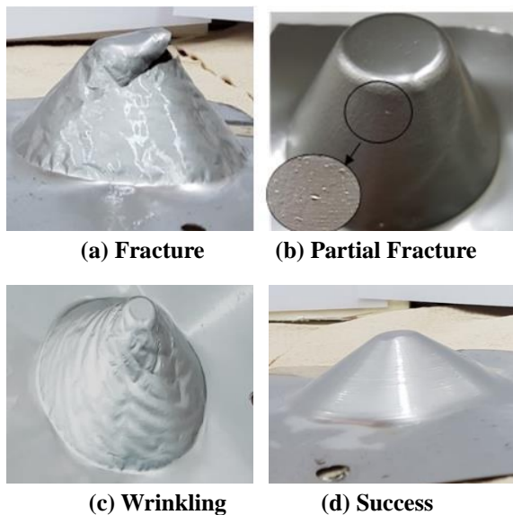
Fig. 3 Classification of Experimental Results: (a) Fracture (b) Partial Fracture (c) Wrinkling (d) Success
